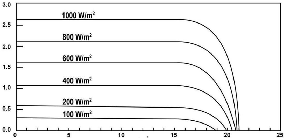
**Figure 3.7:** *Effect of sunlight intensity on module performance (12VDC nominal)*
