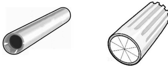
**Figure 10.4:** *Wire to wire connectors*
