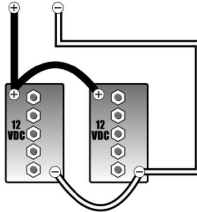
**Figure 4.2:** 12-volt battery configurations
