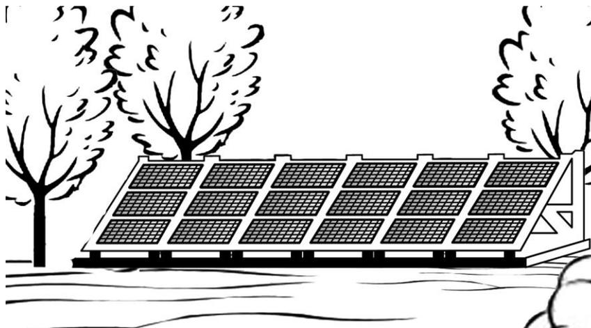
**Figure 10.2:** Ground mounting system
