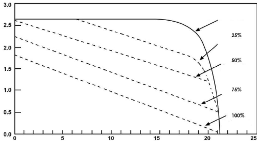
**Figure 3.9:** Effect of shading on module performance (12VDC nominal)
