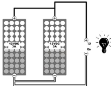
**Figure 3.4:** PV modules in parallel
