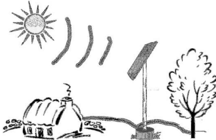
**Figure 10.1:** Pole mounting system
