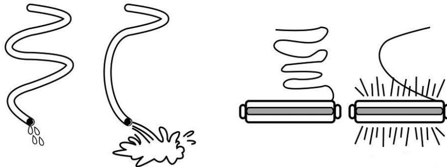
**Figure 7.2:** *Effect of length on power loss*
