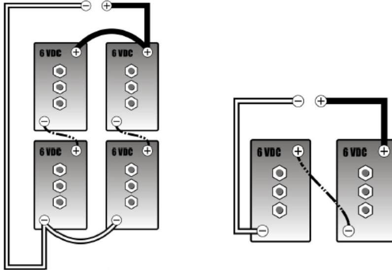
**Figure 4.4:** 48-volt battery configurations
