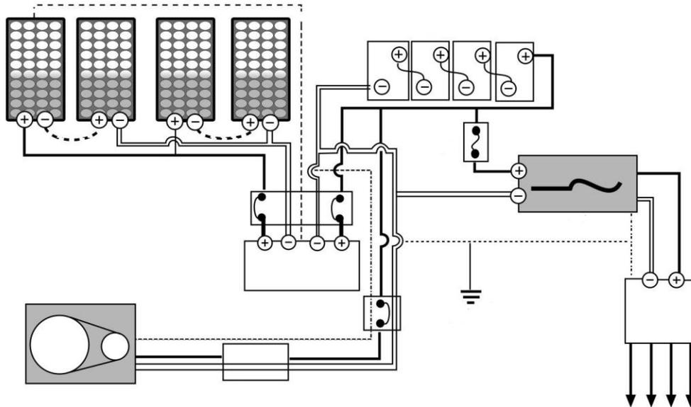
**Figure 9.3:** Hybrid system with generator
