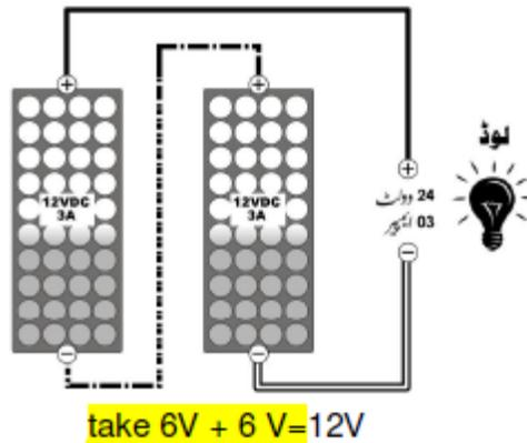
**Figure 3.3:** PV modules in series
