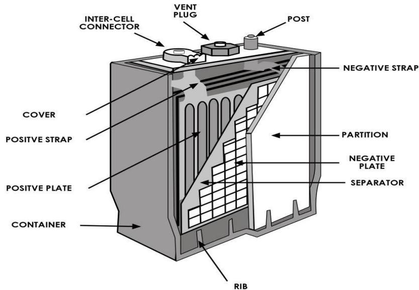
**Figure 4.1:** *Cut-away of a standard lead acid battery cell*
