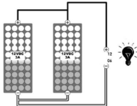
**Figure 3.4:** PV modules in parallel
