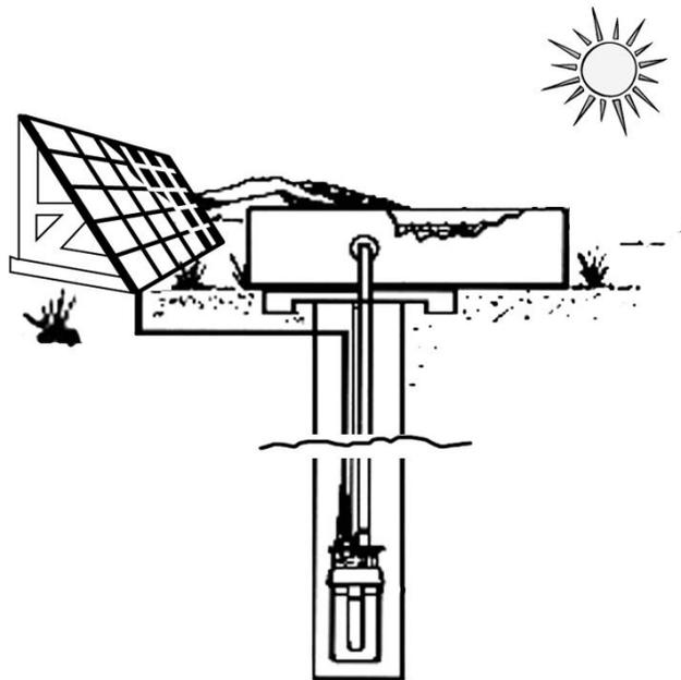
**Figure 9.2:** *Solar water pumping system*
