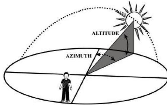
**Figure 2.1:** Azimuth and altitude for all northern latitudes
