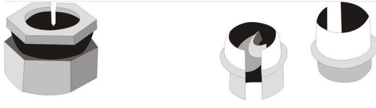
**Figure 10.6:** *Wire to electrical box connectors*
