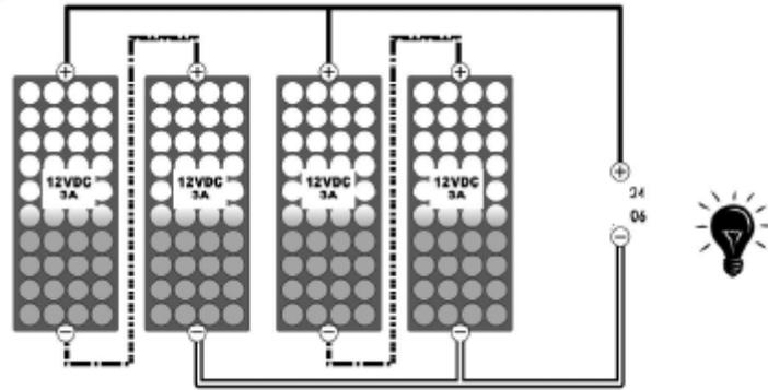
**Figure 3.5:** PV modules in series and parallel
