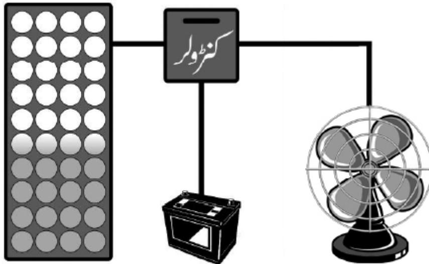
**Figure 5.1:** *Controller in a PV system*
