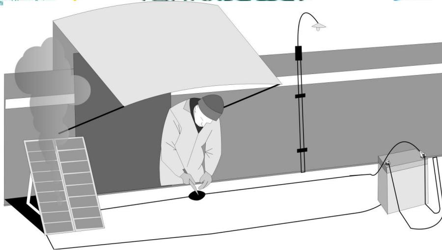
*Do not remove the blocking diode between the solar panel and the battery; it will damage your panel by reverse current flow.*
