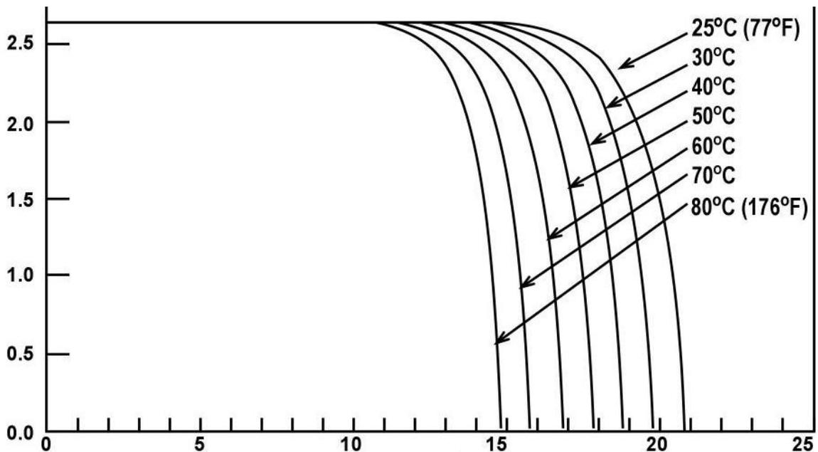
**Figure 3.8:** *Effect of cell temperature on module performance (12VDC nominal)*
