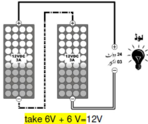
**Figure 3.3:** PV modules in series
