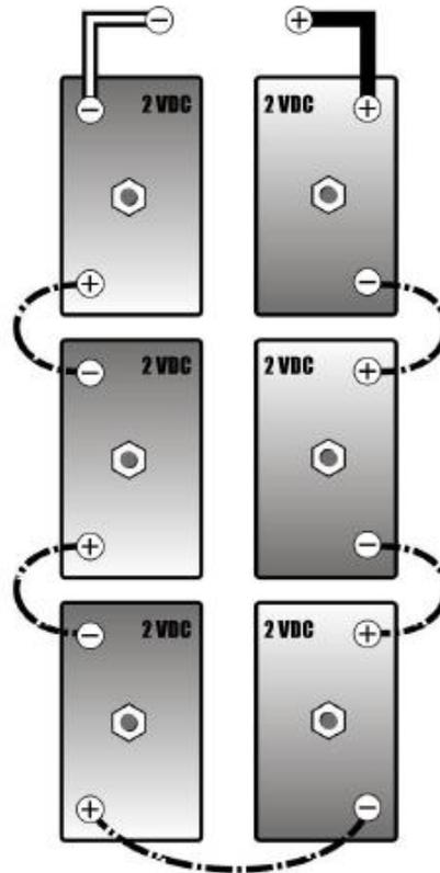
**Figure 4.3:** 24-volt battery configurations
