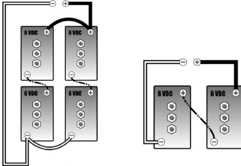
**Figure 4.4:** 48-volt battery configurations
